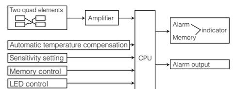
TAKEX original CPU controls all of sensor functions including signal processing and calculation work.
