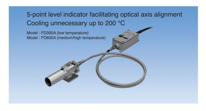
The optical head and amplifier are connected with a fiber optic cable and the infrared ray captured with the optical head is transmitted through highly transmissive glass fiber into an amplifier installed at a distant location. The infrared ray transmitted into the amplifier is optically converted in the light sensitive element and amplified for control signal output (mini power relay, signal relay or solid state output).
