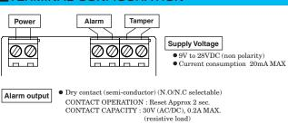
CONTACT CAPACITY: 30V (AC/DC), 0.1A MAX.
