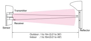
\* Protection distance (between sensor/reflector) should be set in the rated range
