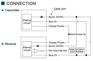
The sensors are supplied in coordinated pairs of an ultrasonic transmitter and a receiver each of which has a matching serial No.
