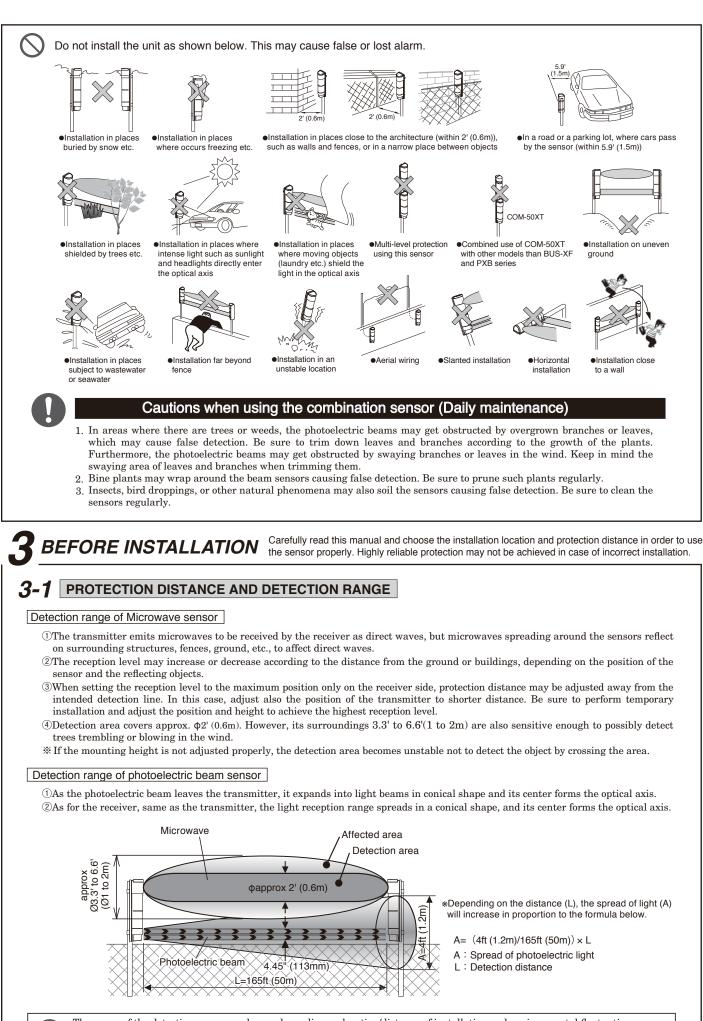
The range of the detection area may change depending on location/distance of installation and environmental fluctuation. Use the above just as reference. If the mounting position/height are not optimal, the detection area may become wider than 2 m, and there will be more risk of malfunctions due to movement of trees and cars around the area.
