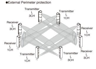
Install the sensors so that only transmitters or receivers come at the corner. Same Modulation frequency can be used in this installation. Straight Line Protection
