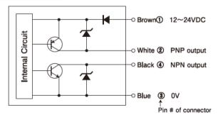
Loaded short circuit or overload shuts off the output transistor. Turn the power back on after checking the loaded condition.
