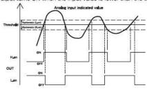
In Han mode, hysteresis subtracted from the threshold (ON point) will be the OFF point. (ex. Threshold (ON point) **300** - Hysteresis **0.50** = OFF point 2.50) In Lan mode, hysteresis plus the threshold (ON point) will be the OFF point.
