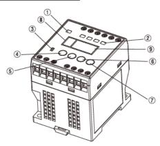
DMC-A4A is an analog comparator which compares analog input with a threshold and generates an open collector output according to a preset logic. Threshold and hysterisis are freely set for each of the four outputs.
