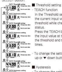
In the Threshold setting mode for OUT1-4. the current input value can be set as the threshold while checking the operating status.
