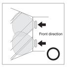
If the sensor mounted on a high ceiling cannot cover the whole glass surface, add additional sensors to a wall surface also.
