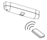
(3) Activate the glass checker by pointing its transmission section toward the sensor unit from the glass surface to be protected, and check the sensitivity. Check it from all the positions of the glass surface to be protected.
