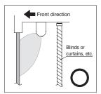
Mount the sensor between the glass and the blind or curtain.
