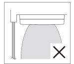
Mount the front of the sensor (indicated by 'Front mark') facing the glass surface.
