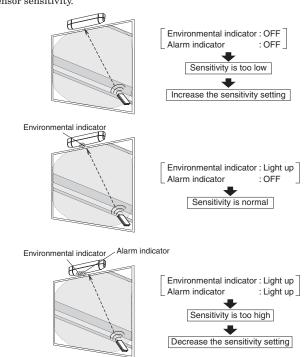
(5) If detection operation has not been performed for approximately five minutes after the sensitivity check finishes, the mode automatically switches to "Operation mode". Check that the alarm indicator is not blinking before operation.
