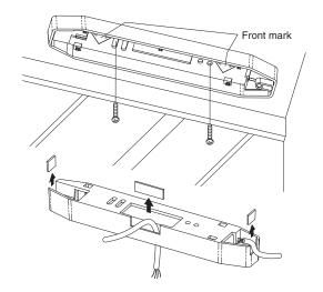
3. Connect the wires to the terminal block on the sensor unit. As an extra terminal is reserved for interconnected wiring, make sure to connect only one electric cable to one pole on the terminal block.
