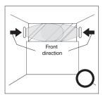
When protecting a long, horizontal glass surface, you can mount two sensors facing each other on the wall surfaces at both ends.
