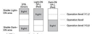
The red LED is an operation indicator. For Light On Type, it will light when the beam goes through. For Dark On Type, it will light when the beam is interrupted.
