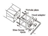
Mount the pinhole plate on sensor with hood.
