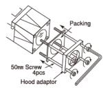
(The tighting torque of the bolt should be less than 0.8N·m.)
