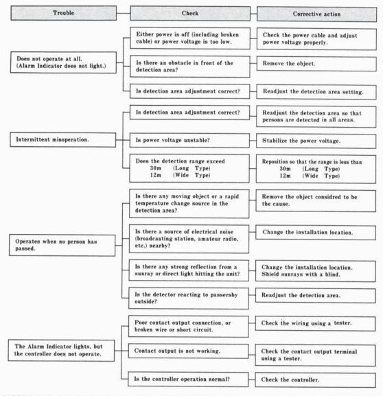
The PASSIVE INFRARED SENSOR is designed to detect infrared energy variations caused by the presence of a human body. Therefore, note that similar variations in conditions in protected area, due to other reasons, may cause the sensor to create an alarm as it is unable to distinguish between sources.
