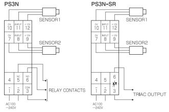
A short bar is attached to the terminal #7 and #8. Take off the short bar when AND mode is selected, and connect sensor #2.
