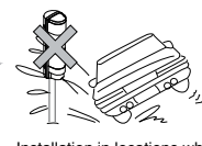
• Installation in locations where the device may be splashed by dirty water or direct sea spray.
