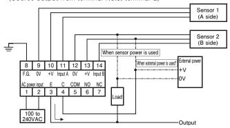
\*Since the open collector output is isolated with a photocoupler, if desired an independent external power supply can be used.
