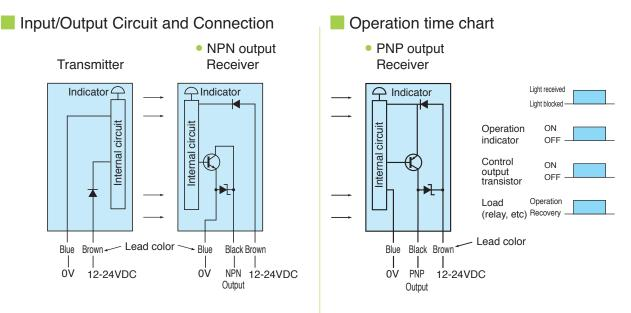
The output transistor turns off when load short circuits or overload occurs. Check the load and turn the power back on.
