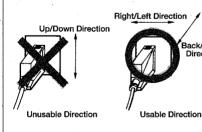
※ Unusable direction to use Take care for the up/down direction as like above picture except for the detection range, because it's impossible direction to use.
