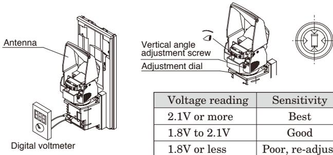
After adjustment, set the adjustment mode switch to "Operation mode".
