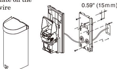
\*The grommet is compatible with a wire of  $\phi 0.12"$  ( $\phi 3\text{mm}$ ) to  $\phi 0.24"$  ( $\phi 6\text{mm}$ ) outer diameter. When a wire of more than  $\phi 0.24"$  ( $\phi 6\text{mm}$ ) outer dia. is used, cut off the dotted line portion as illustrated using pliers or the like. Then use caulking to prevent insects from entering into unit.
