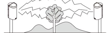
Note: Install the sensor at a proper height and position otherwise detection area could be widened over 6.6' (2m). This could cause the sensor to detect movements of cars or vegetations near the area and lead to frequent false alarms.
