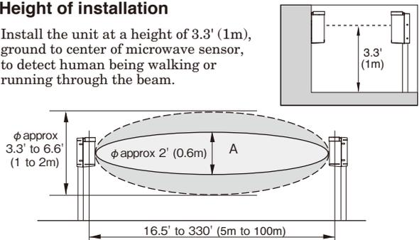
A core detection area is approximately φ 2' (0.6m) as indicated above as A, when the alignment is correctly adjusted. It is suggested to make at least 3.3' (1m) open space on either side of detection area to prevent false alarm.
