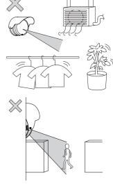
Remove objects including clear glass which would block the infrared ray and create no detection zone.
