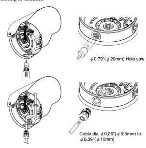
\*\*Please apply sealing materials to the screws and wiring hole to prevent water from entering.
