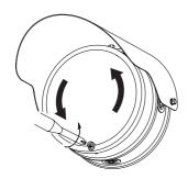
2. Loosen inside sensor locking screws (2pcs) and detach the base from the sensor body.
