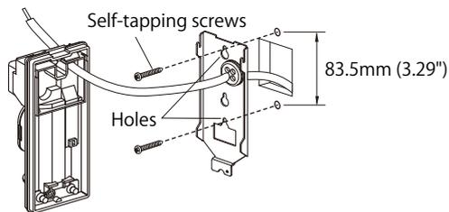
Pull the wire through the sensor body (back to front) and attach it to the terminals on the sensor.
