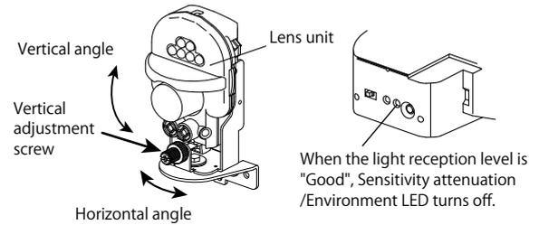
When the direction of the optical axis roughly matches the reflector, a beep sound begins which changes according to the light reception level as below.
