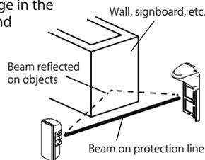
In "Normal" mode, lost alarm caused by light wraparound can be prevented by monitoring these two changes.
