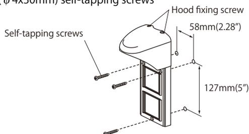
※In case of indoor installation, the hood can be removed if it is not required.
