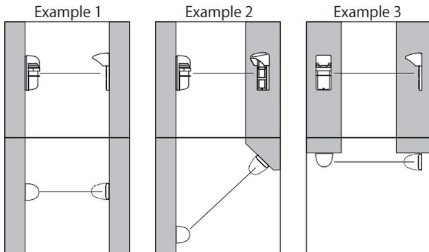
Install the reflector directly, facing the front of the optical unit as much as possible. Reflection efficiency of the reflector, due to its nature, decreases as the angle from the directly facing position increases. Make sure that angle remains within  $\pm 15^\circ$  even if angled installation is needed. When exceeding this, the amount of reflected light will be insufficient and it will not operate correctly.
