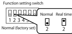
③ Response time adjustment (Function setting switch: DIP 3/4)
