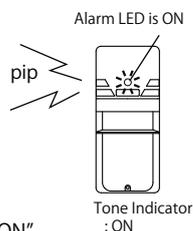
※When setting tone indicator to "ON", walk test mode starts 5 minutes after closing the cover, and pip sound comes out for alarm.
