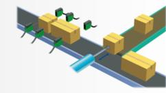
Several sensors are used to identify the length of carton boxes.
