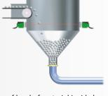
Detection of level of material inside hopper.
