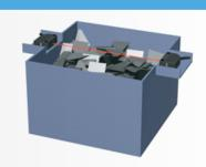
Press cuttings detected as they fill the container. Note: Separate SUS protective covers are available.
