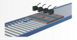
Pallet checked for any missing tile. Reliable detection is achieved without being affected by tile color variation.
