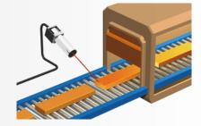
Detecting the presence of material at the outlet of furnace. The detecting head is highly heat-resistant.
