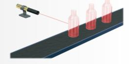
HMD used for the detection of hot formed bottles.
