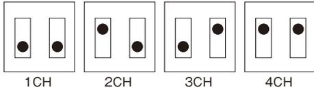
MAKE SURE TRANSMITTER AND RECEIVER OF PAIR ARE SET AT SAME CHANNEL ! Paired TR/RE will not set up unless set at the same channel.
