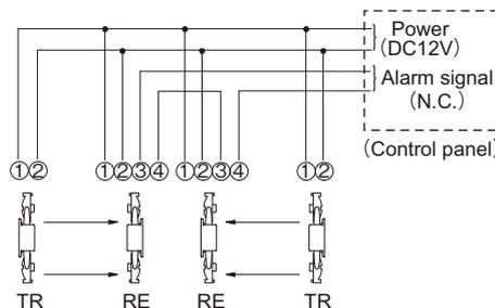
**3) When two or more sensors are connected to separate lines.**
