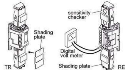
After initial beam alignment is completed, definitive alignment is achieved by using a voltmeter.
